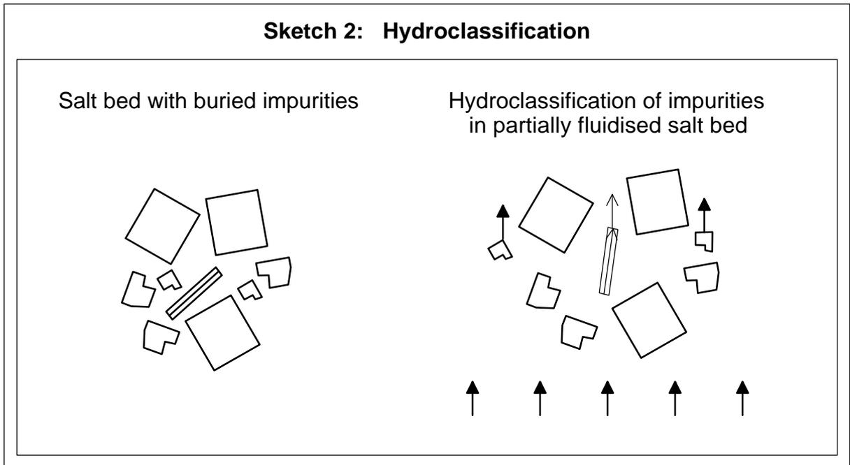
upwards out of the salt and to the overflow of the process vessels. The brine velocity is
