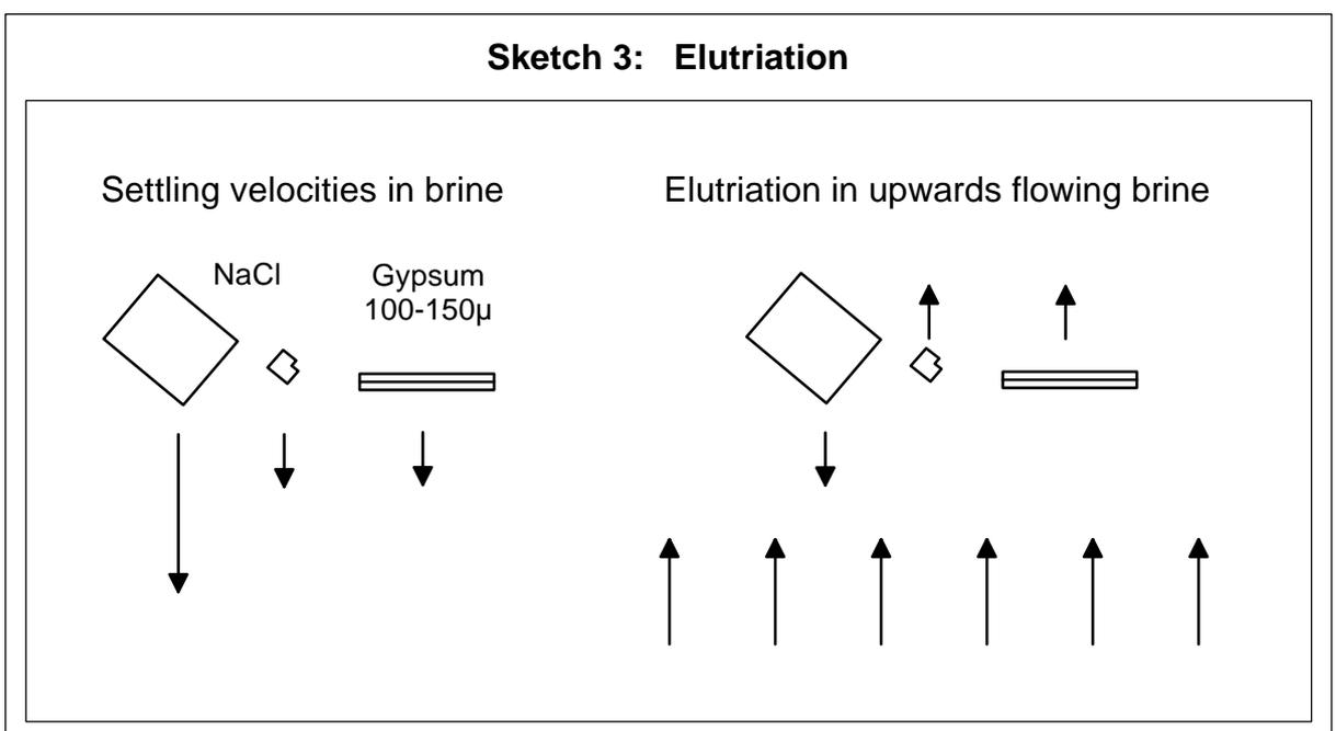
precisely controlled to remove just the right size of particles containing as much impurities as possible but very little salt. This is called elutriation and hydroclassification.
